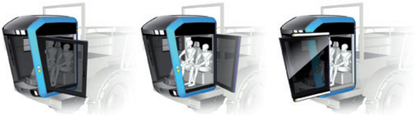
An example of AgriCab's flexibility: the same cabin can be equipped with a conventional door, a rear-hinged door or a sliding door, all to suit each customer's needs.
