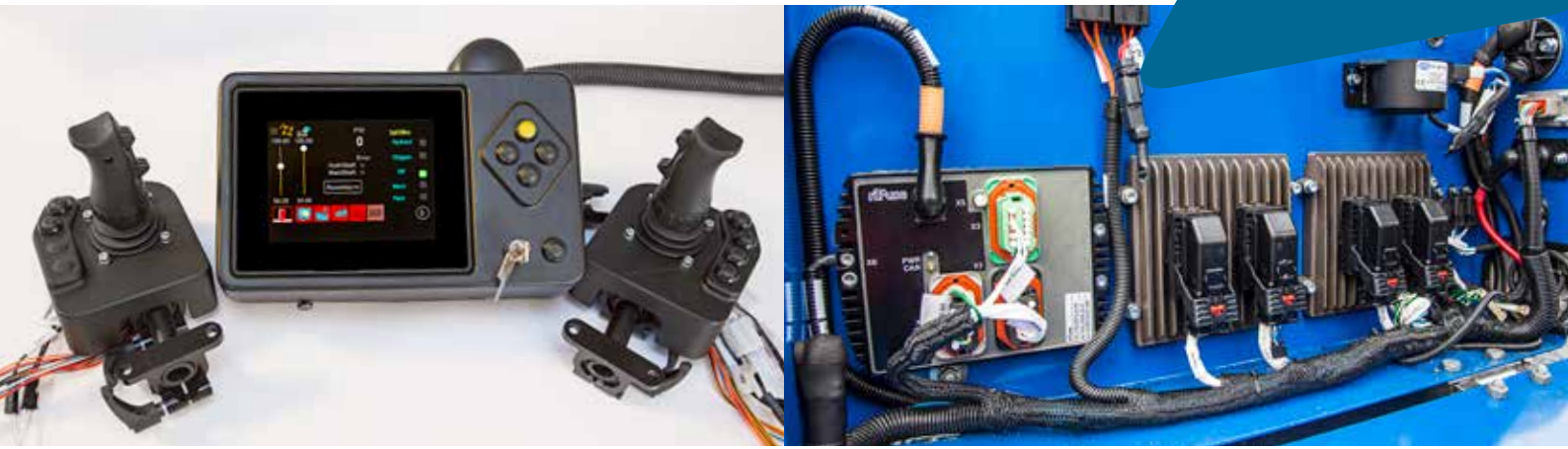
Rimaster consoles with mounted Parker IQAN LC6 joysticks as well as a Rimaster display unit including a Parker IQAN MD5 display. The image to the right shows the power plant, including the Rimaster riFuse unit, which eliminates fuses and relays, as well as Parker IQAN modules.
